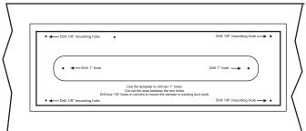
2. Drill two 1" holes and four 1/8" mounting holes as noted on the template.
