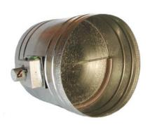
The POC is designed for the jobs that need both power open and power closed dampers. With the high torque motor it operates very well in the 2,000 fpm range. For use in residences, industrial buildings, schools, theaters and public buildings, etc. They have been tested at over 2,000 cfm and thousands of cycles without failure.
